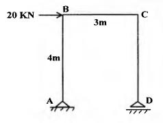
Q.3 (b) For the pin jointed frame loaded as shown in figure below, find the vertical (10) deflection of joint C.
